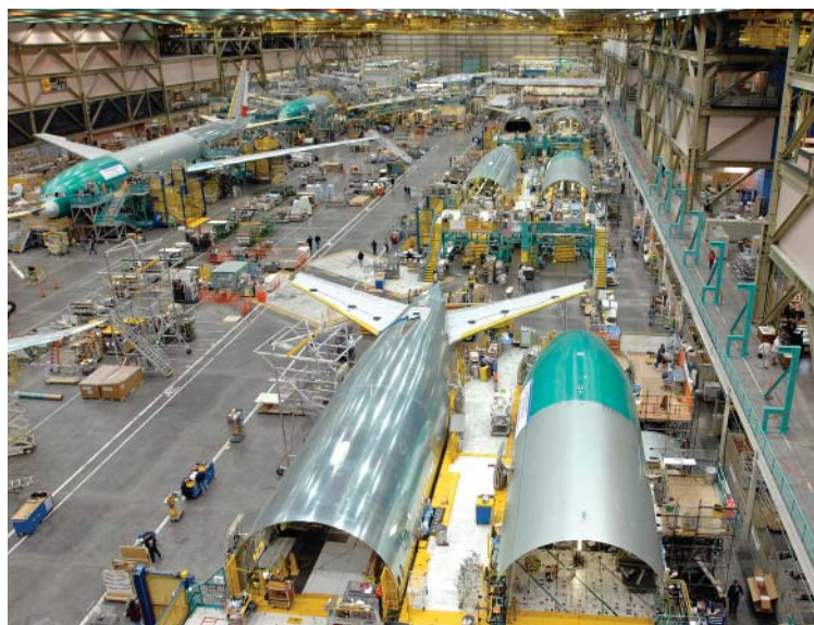
The 777 moving line, which will be complete in 2008, includes systems installation, final body join and final assembly. With implementation of the Boeing Production System, Boeing has made significant improvements to 777 manufacturing, including reduction of factory flow time for the airplane, increased inventory turns and improved quality. A continued focus on Lean will create opportunities for further improvements.
