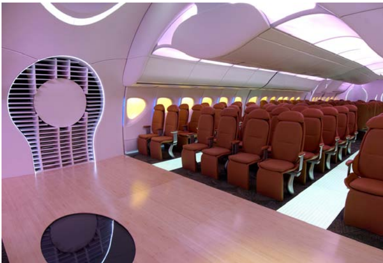
Interior View – D-shaped windows, new overhead design and a floor display (foreground) for viewing the terrain below are features of a next-generation airplane cabin mockup at Boeing's ConceptCenter in Everett, Washington.
