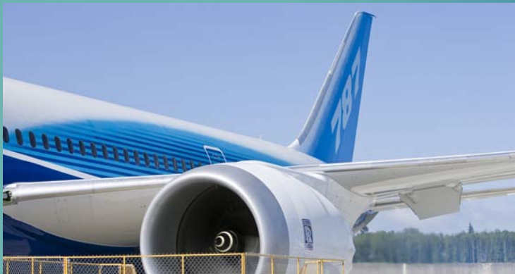
Engine runs begin – The 787's first engine runs marked the first all-electric start of a commercial jetliner engine onboard a twin-aisle commercial jetliner.
