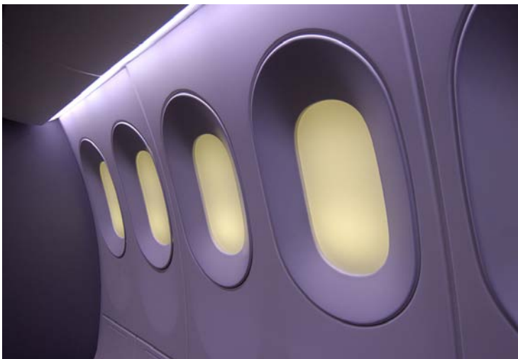
Cabin advances – Dimmable windows and LED lighting are among technology breakthroughs incorporated into the new 787.
